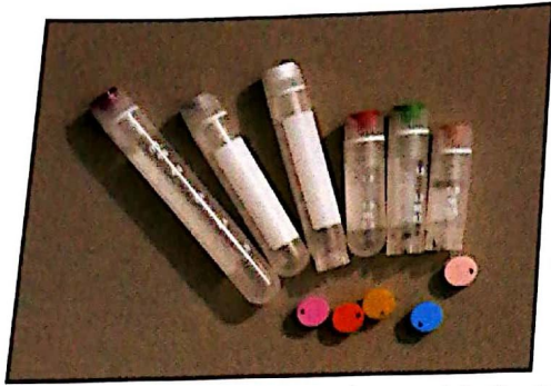
(d) Color-coded Cryovials. Polypropylene cryovials of various sizes, ranging from 1.0 to 4.6 mL. Colored inserts can be added to the caps to help identify cryovials. Source: Courtesy of Alpha Laboratories.
