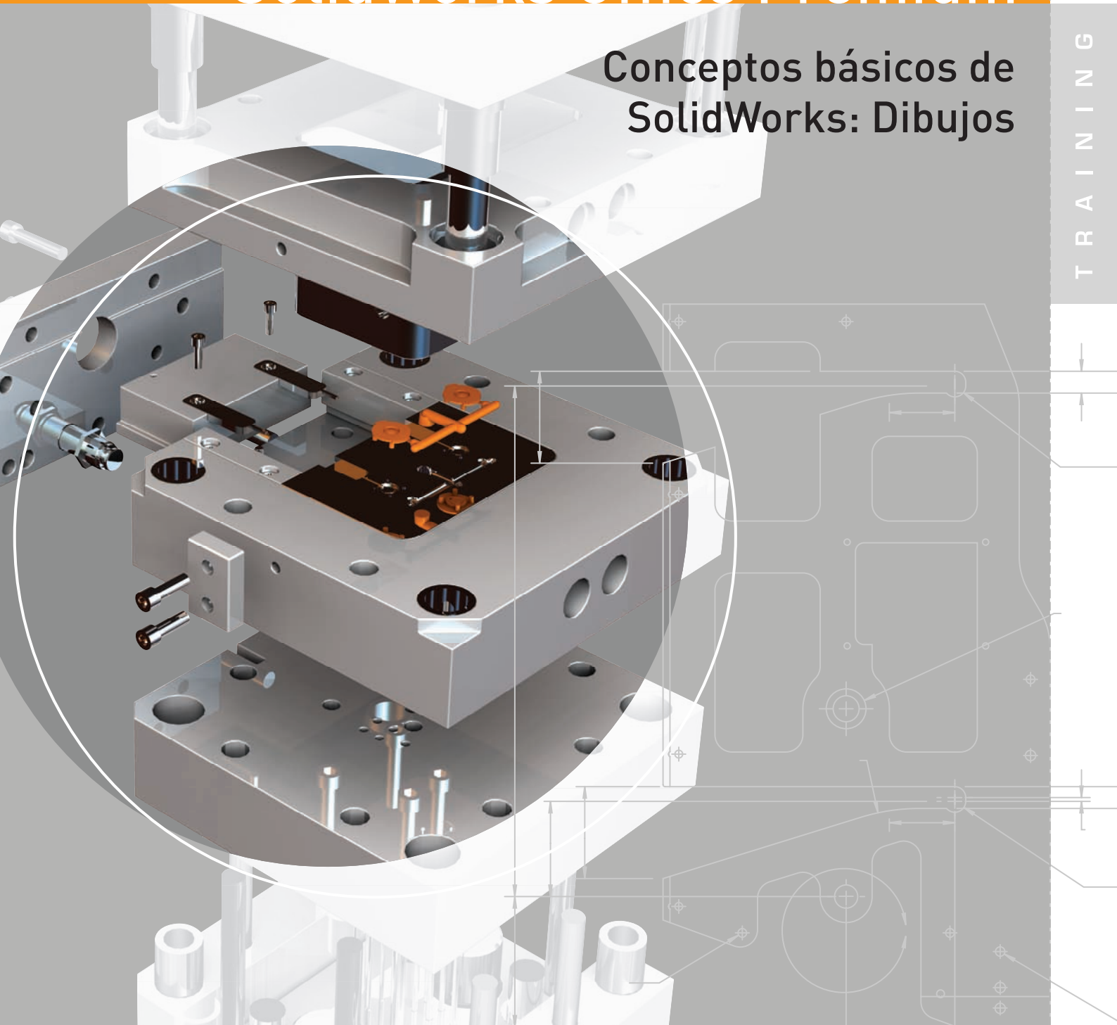
Image of 2-Cavity Mold for Valve Cap courtesy of JK Mold Design
